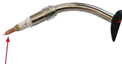
(16) Fit an Aluminium contact tip of the correct size to match the wire diameter being used
