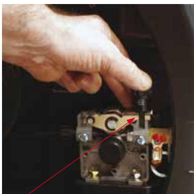
(9) Close down the top roller bracket and clip the pressure arm into place.
