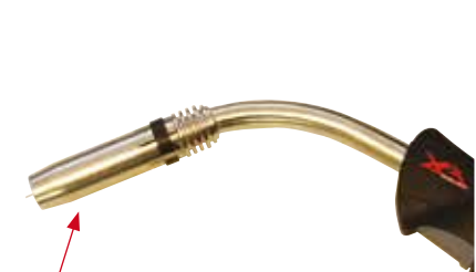
(14) Fit the nozzle to the torch head.
