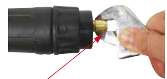
(9) Fully screw down the liner retaining nut and nip it up tight.
