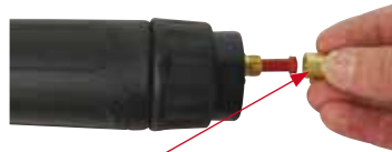
(2) Remove the liner retaining nut
