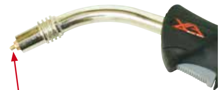
(6) Replace the front end parts
