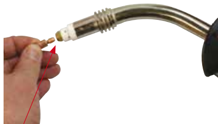
(10) Remove the gas nozzle and contact tip from the front end of the mig torch.
