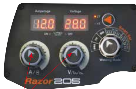
(16) Set welding parameters using the wire feed and voltage knobs.
