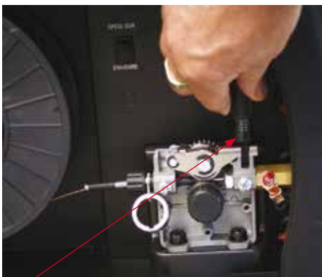
(9) Close down the top roller bracket and clip the pressure arm into place with a medium amount of pressure applied.
