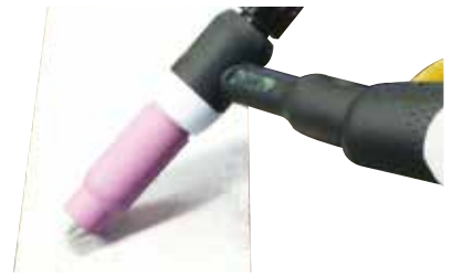
(10) Lay the outside edge of the Gas Cup on the work piece with the Tungsten Electrode 1- 2mm from the work piece. Press and hold the trigger button on TIG torch to start the gas flow.
