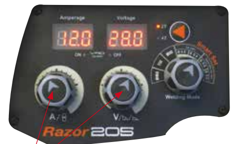
(17) Set welding amperage using the wire feed knob, increasing the wire feed increase the amperage. Fine tune if required using the voltage knob.
