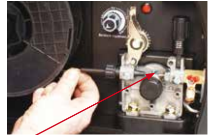
(7) Place aluminium wire onto spool holder. Feed the wire through the inlet guide tube on to the drive roller.
