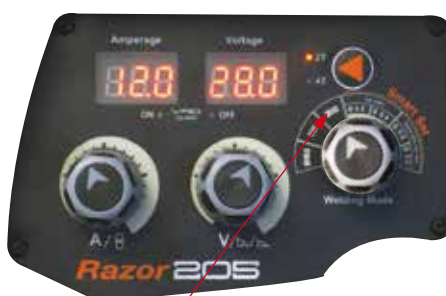
(18) Select MIG function and 2 or 4T trigger Important: Smart Set programs are for solid steel wire only.
