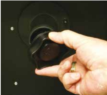
(1) Remove the spool retaining nut.
