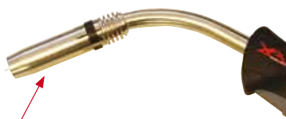
(13) Fit the gas nozzle to the torch head.
