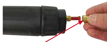
(2) Remove the liner retaining nut
