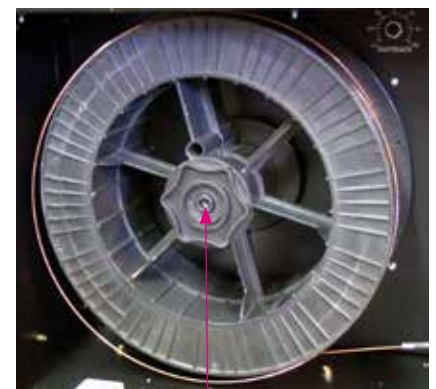
(8) The weight and speed of the wire spool turning creates an inertia that can cause the spool to run on and the wire loop over the side of the spool and tangle. If this happens increase the pressure on the tension spring inside the spool holder assembly using the tension adjustment screw.
