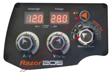
(7) Select TIG function, 2T, 4T Trigger as required
