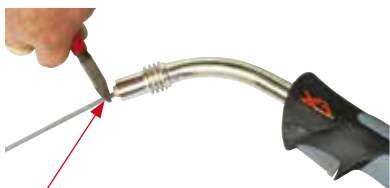
(7) Snip the liner off 3mm past the end of the torch neck.
