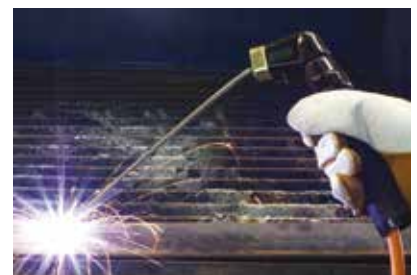
5) Strike the electrode against the work piece to create an arc and hold the electrode steady to maintain the arc
