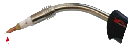
(13) Fit the correct size contact tip over the wire and fasten tightly into the tip holder.
