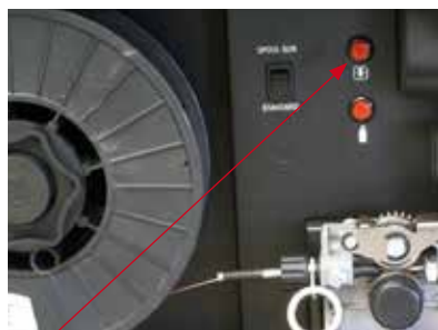
(12) Press and hold the inch wire button to feed the wire down the torch cable through to the torch head.
