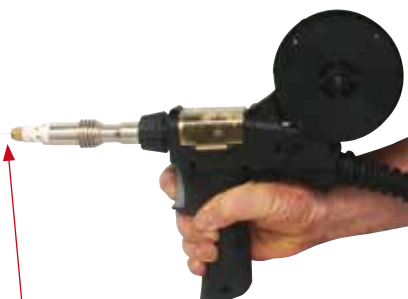
(14) Remove the gas nozzle and contact tip. Pull the trigger to drive the wire through the neck until it exits the contact tip holder
