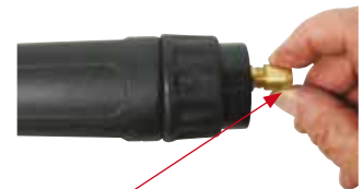
(6) Fit the liner retaining nut and screw down only 1/2 way down
