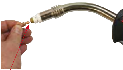
(11) Remove the gas nozzle and contact tip from the front end of the mig torch.
