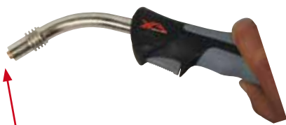
(1) Remove mig torch front end parts
