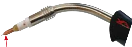
(12) Fit the correct size contact tip over the wire and fasten tightly into the tip holder.
