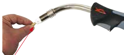
(8) Replace the front end parts
