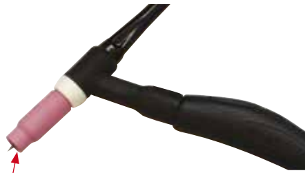
(9) Assemble front end parts of the TIG torch, fitting a sharpened tungsten suitable for DC welding.
