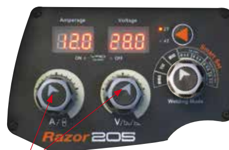
(19) Set welding parameters using the wire feed and voltage knobs.
