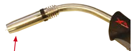
(17) Fit the remaining front end parts to the torch neck ready for welding.
